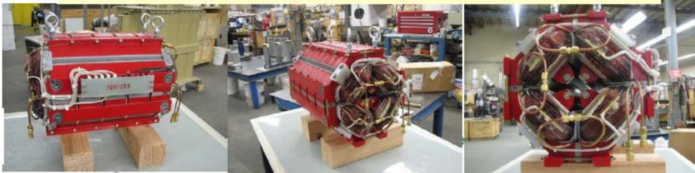
Beam Transport Quadrupole Magnets (50 of 114 total) at JLab
